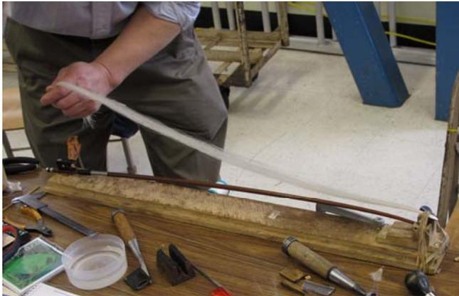
Once it was combed out, Jon repeated the process of tying, heating and rosinning the frog end of the hair. The trick here is to know how long to make the hair so it will not be too tight or too slack, as heat and humidity change. To me this seemed the part requiring the most experience.
